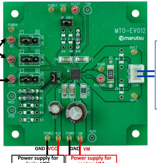
Power supply for logic: VCC (3.0V to 5.5V) Power supply for motor: VM (4.5V to 38V)
