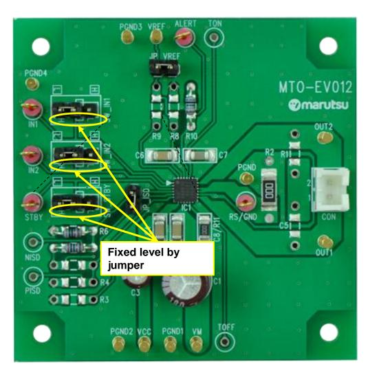
Jumper indicated on the left is adopted on this evaluation board to set operation of the TB67H301FTG. In the left figure, fixed level of the silk near the jumper is indicated inside the white frame. Please change the short position according to the configuration of the usage function. In case of inputting the signal externally, please remove the short pin.
