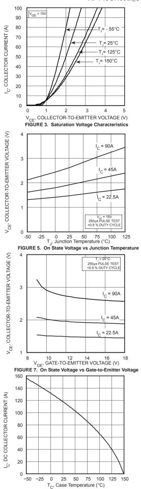
FIGURE 9. DC Collector Current vs Case Temperature
