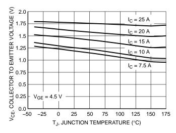
Figure 3. Collector-to-Emitter Voltage vs.
