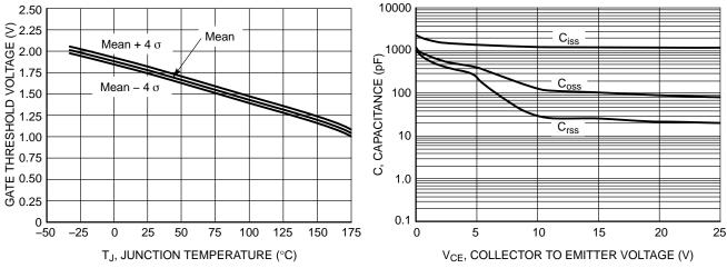
Figure 9. Gate Threshold Voltage vs. Temperature
