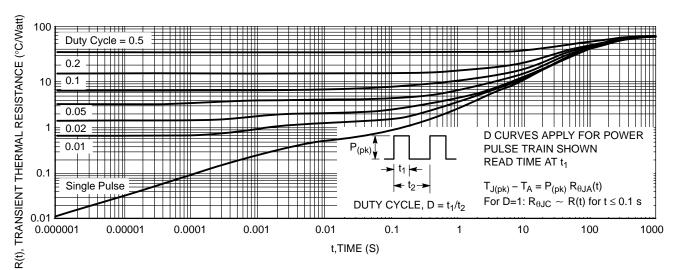
Figure 13. Minimum Pad Transient Thermal Resistance (Non-normalized Junction-to-Ambient)
