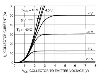
Figure 6. Collector Current vs. Collector-to-Emitter Voltage
