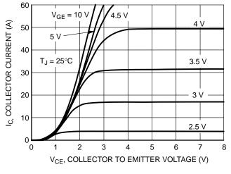
Figure 5. Collector Current vs. Collector-to-Emitter Voltage
