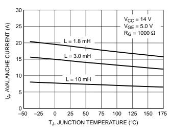
Figure 2. Open Secondary Avalanche Current vs. Temperature
