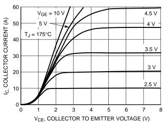
Figure 4. Collector Current vs. Collector-to-Emitter Voltage
