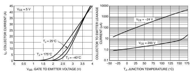
Figure 7. Transfer Characteristics
