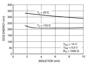
Figure 1. Self Clamped Inductive Switching
