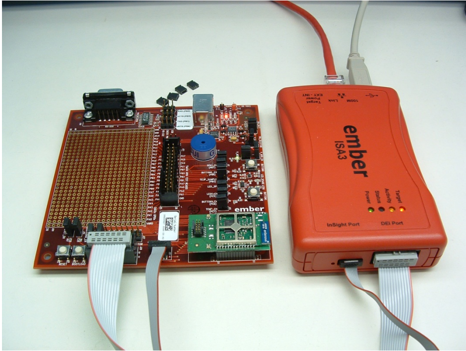
Figure 4-7. ISA supplying power; RS-232 serial communication
