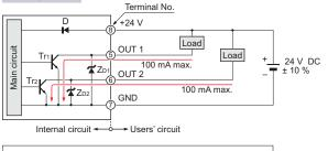
Symbols ... D: Reverse supply polarity protection diode ZD1, ZD2: Surge absorption zener diode Tr1, Tr2: NPN output transistor
