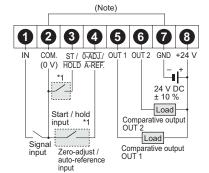
Note: COM. (0 V) is internally connected to GND.
